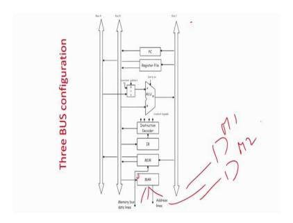
Because if there is a multiple ports over here; so in fact, in this and they connect to different bus to different lines to the address. So, you should have multiple memory blocks memory 1, memory 2.
